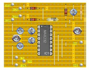
Figure 17 ICOM Component Side
