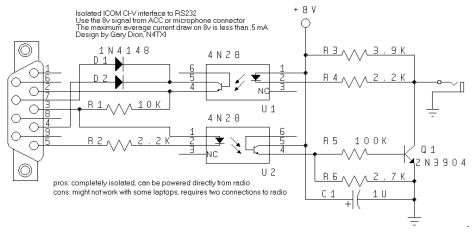
Figure 4: N4TXI opto-isolated circuit
