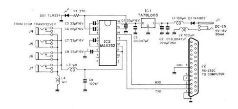
Figure 3: Icom CT-17 circuit
