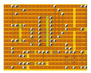
Figure 18 ICOM Solder Side
